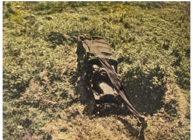
FIGURE 48. A sloped side screen hung from a tree conceals a vehicle from oblique observation. Repairs, unloading, and other activities can be carried on behind it. Camouflage nets used as drapes can often combine the principles shown in figures 47 and 48, and thus provide concealment from both ground and air observation.
